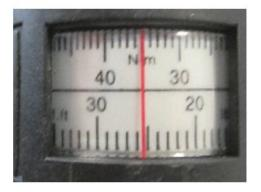
OMB ASSEMBLING PROCESS: PRD is assembled on the valve with a torque value of 35 Nm
